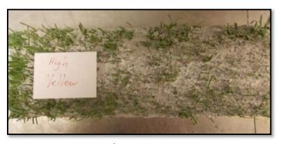
Figure 2. HydroTurf® Post-test Freeze-thaw Sample
