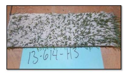
Figure 1. HydroTurf® Pre-test Freeze-thaw Sample
