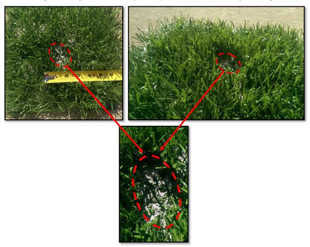
Figure 2. HydroTurf® Sample after Flammability Testing
