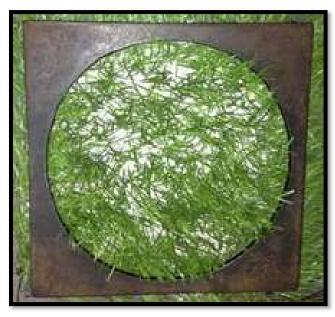
Figure 1. HydroTurf® Sample Prepared for Flammability Testing
