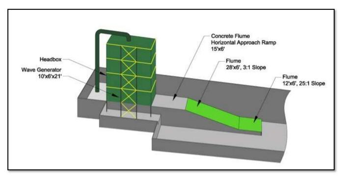
Figure 1. CSU Wave Overtopping Test Facility Diagram
