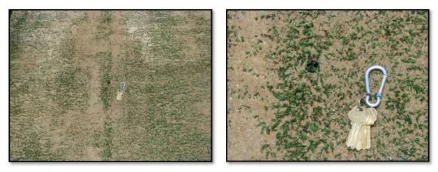
Figure 5. Intentional Damage Simulating a Bullet Hole through HydroTurf®
