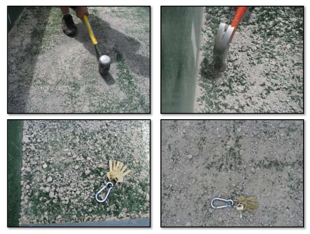
Figure 4. Intentional Damage by Pulverization of HydroBinder<sup>®</sup> Infill
