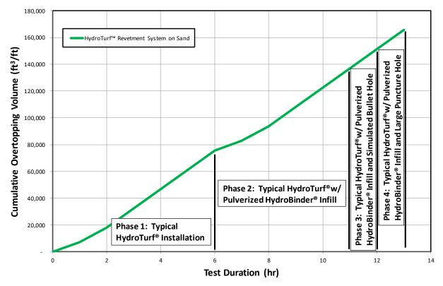
Figure 10. HydroTurf<sup>®</sup> Cumulative Wave Overtopping Volume Progression
