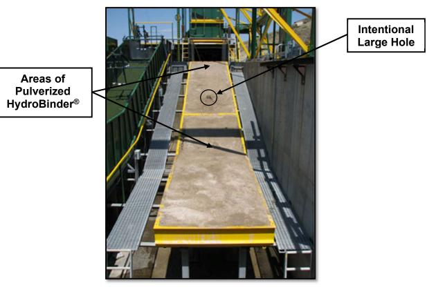
Figure 9. Highly Erodible Silty Sand Subgrade upon Completion of Wave Overtopping Testing
