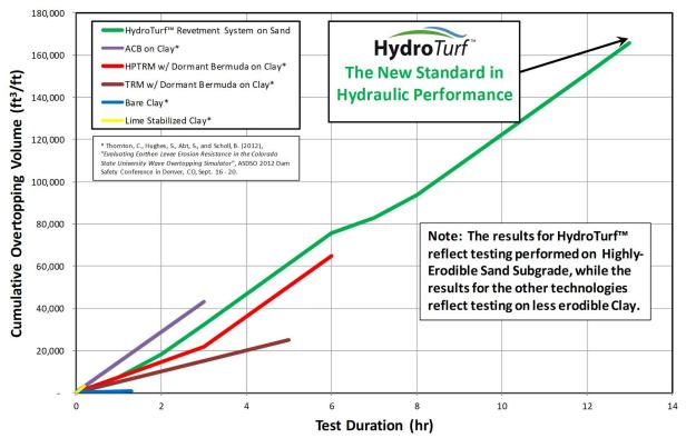
Figure 11. Armoring Performance for Levee Landward-Side Protection from Wave Overtopping
